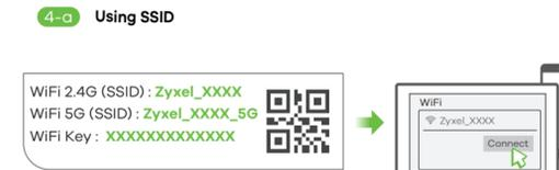
Scan the QR code on the device label to see the SSID and WiFi Key on your smartphone.
