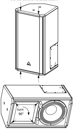
2) Unscrew the 4 screws fixing the horn and rotate the horn by 90°.
