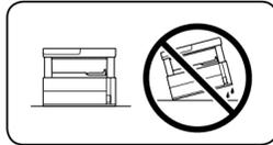
Be sure to keep the ink bottle upright when tightening the cap. Place the printer and the bottle in a plastic bag separately and keep the printer level as you store and transport it. Otherwise ink may leak.
