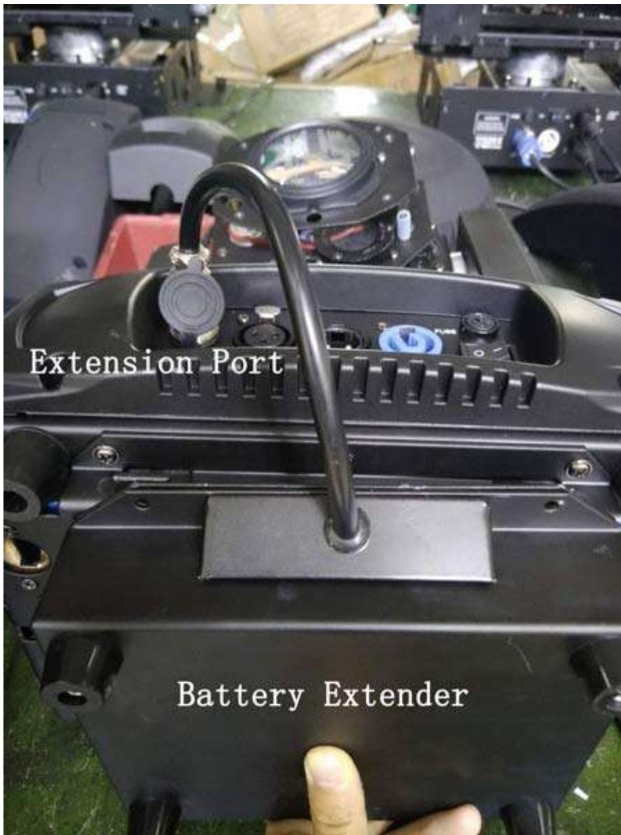
(3). Use Screws to fixed Battery Extender
